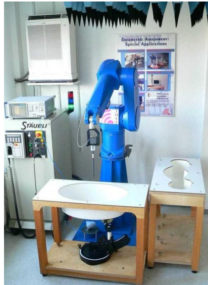
Fig. 3: The measurement set-up with a DASYS system and phantoms containing tissue simulating liquid.
