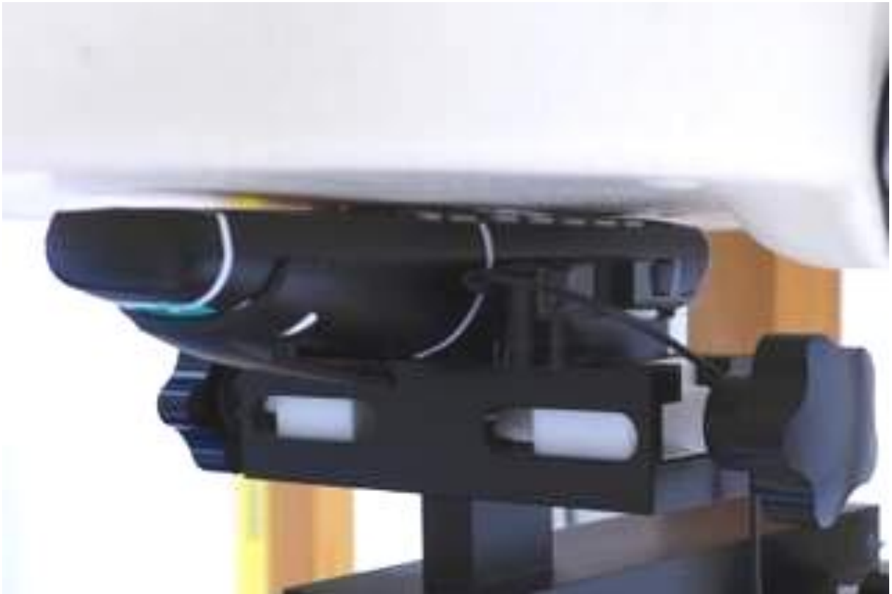
Pic. 8: Body worn configuration, front of the device towards the phantom, 0 mm distance, headset attached.
