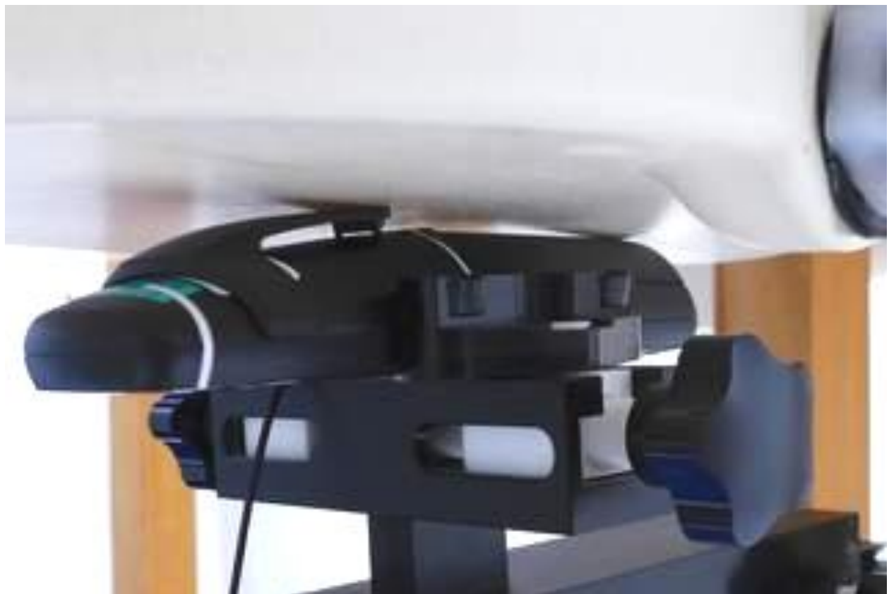
Pic. 9: Body worn configuration, back of the device towards the phantom, 0 mm distance, headset attached.
