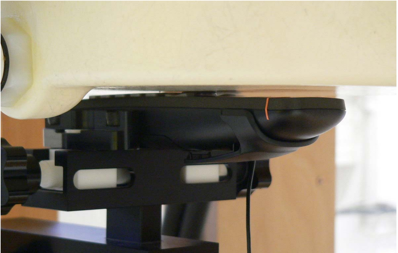
Fig. 18: Body worn configuration for KX-TGFA30, front of the device towards the phantom, headset and belt clip attached, 0 mm distance.
