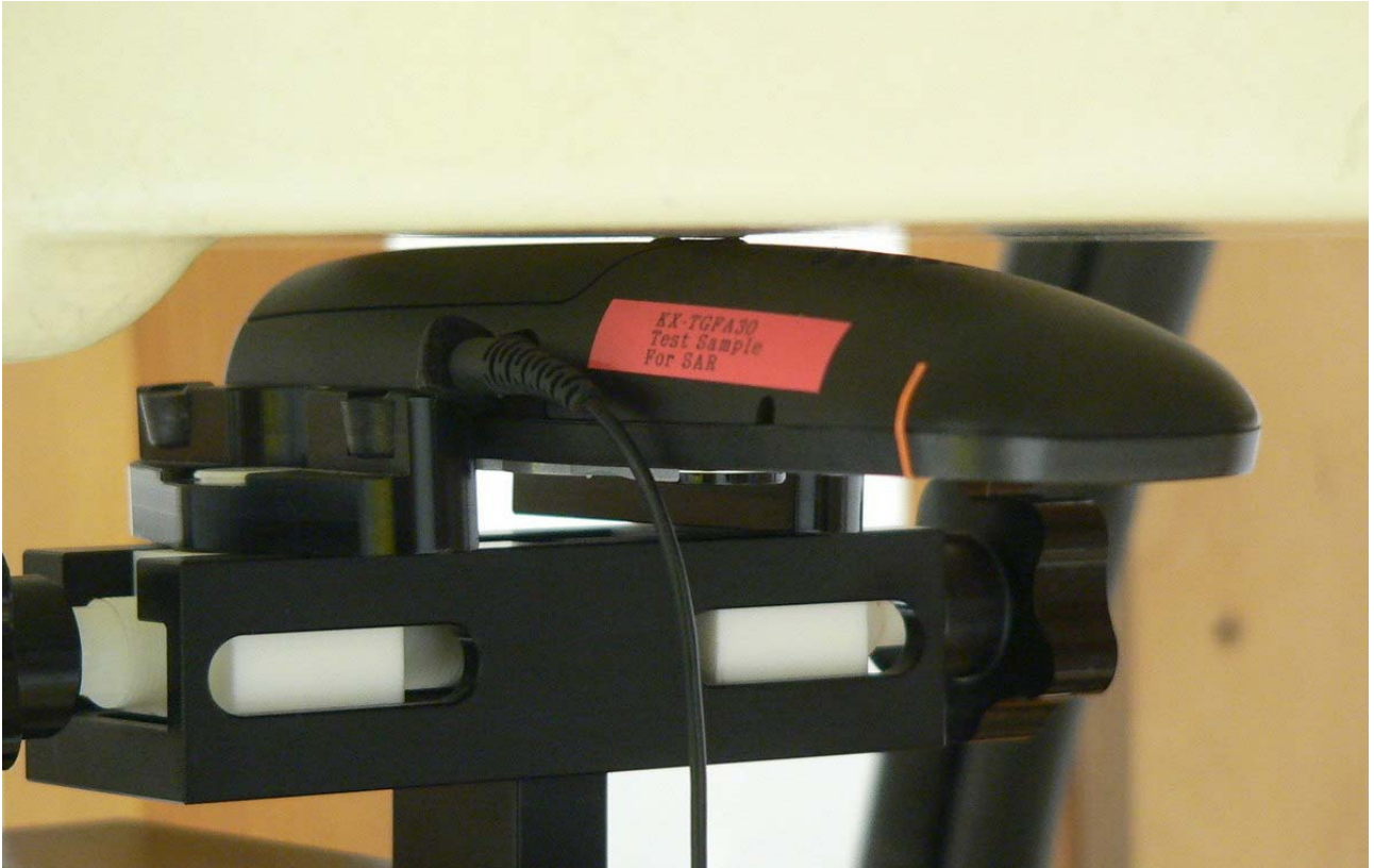
Fig. 19: Body worn configuration for KX-TGFA30, back of the device towards the phantom, headset attached, 0 mm distance.
