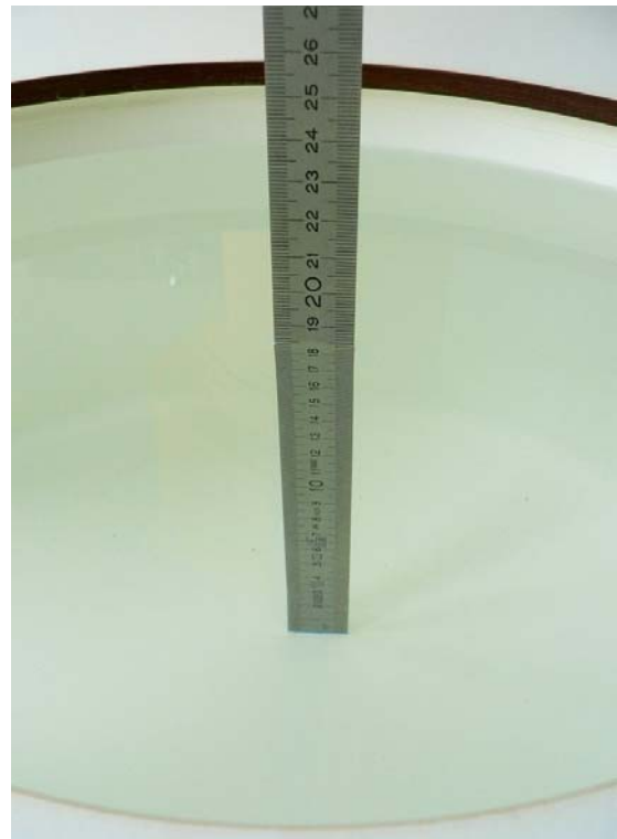
Fig. 21: Liquid depth for 1900 Body worn measurements
