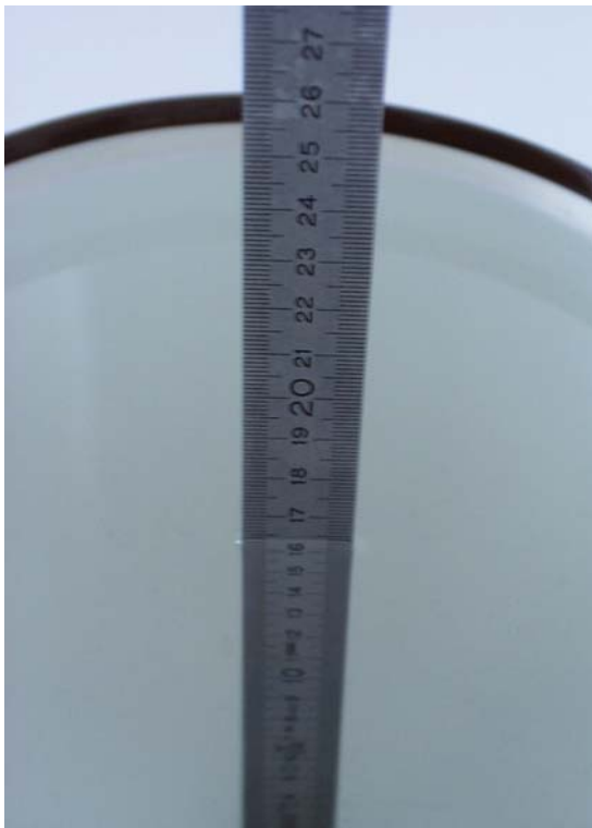
Fig. 20: Liquid depth for 1900 MHz Head measurements
