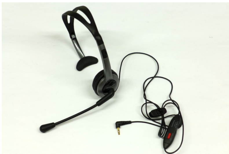
Fig. 13: Pictures of the used headset RP-TCA430.
