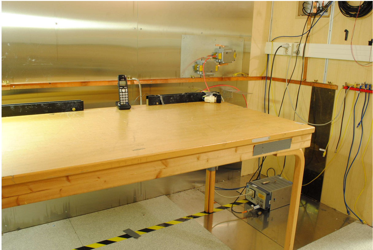
Power line Conducted Emissions Test
