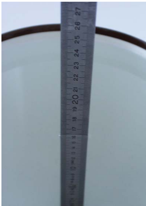
Fig. 16: Liquid depth for 1900 MHz Head measurements
