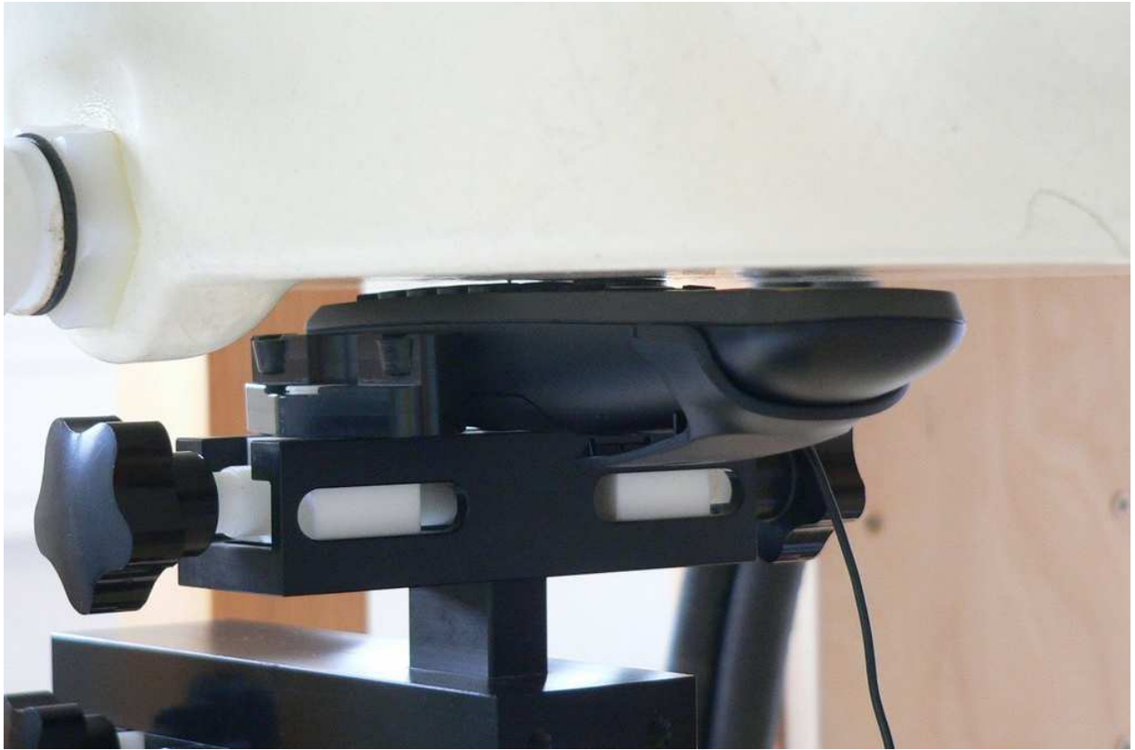
Fig. 19: Body worn configuration for KX-TGA950 with attached belt clip and headset, position 1, display towards the phantom, 0 mm distance.
