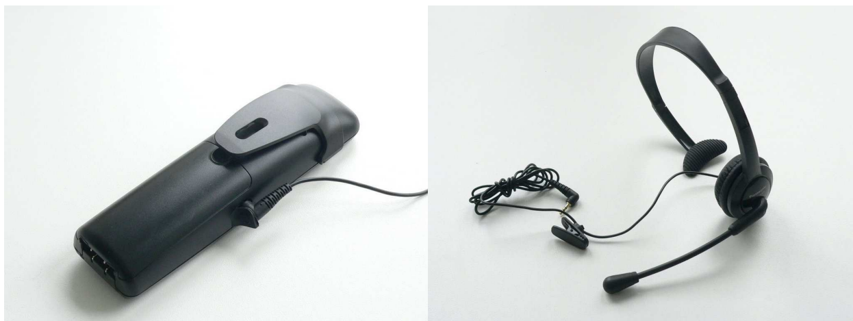
Fig. 14: Pictures of the used accessory for body worn measurements, belt clip and Panasonic TCA-400 headset .
