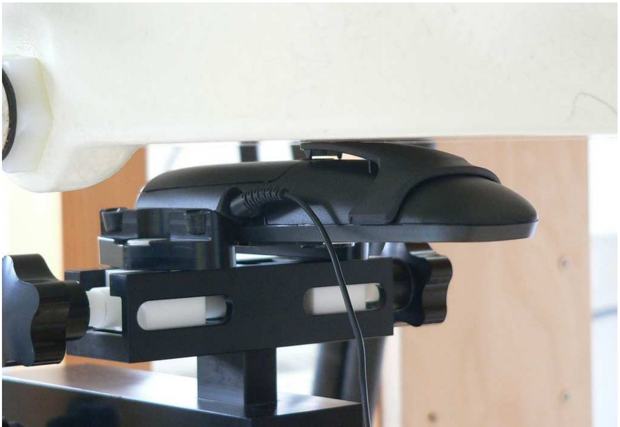
Fig. 20: Body worn configuration for KX-TGA950 with attached belt clip and headset, position 2, display towards the ground, 0 mm distance.
