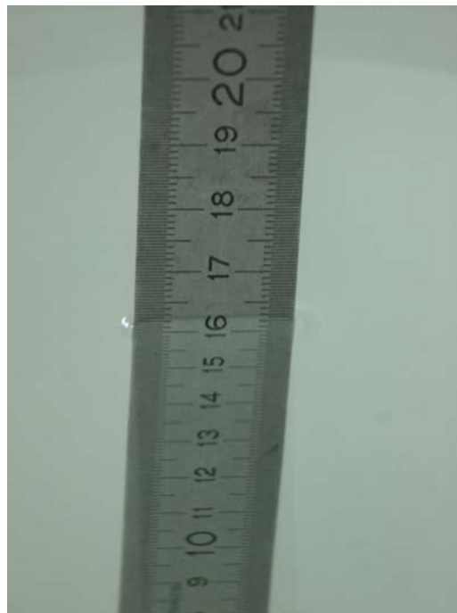
Fig. 23: Liquid depth for the US DECT Body measurements.
