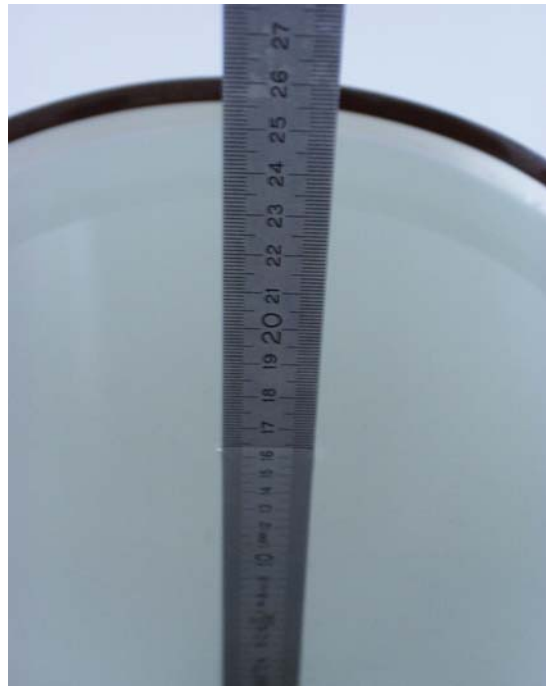
Fig. 22: Liquid depth for the US DECT Head measurements.
