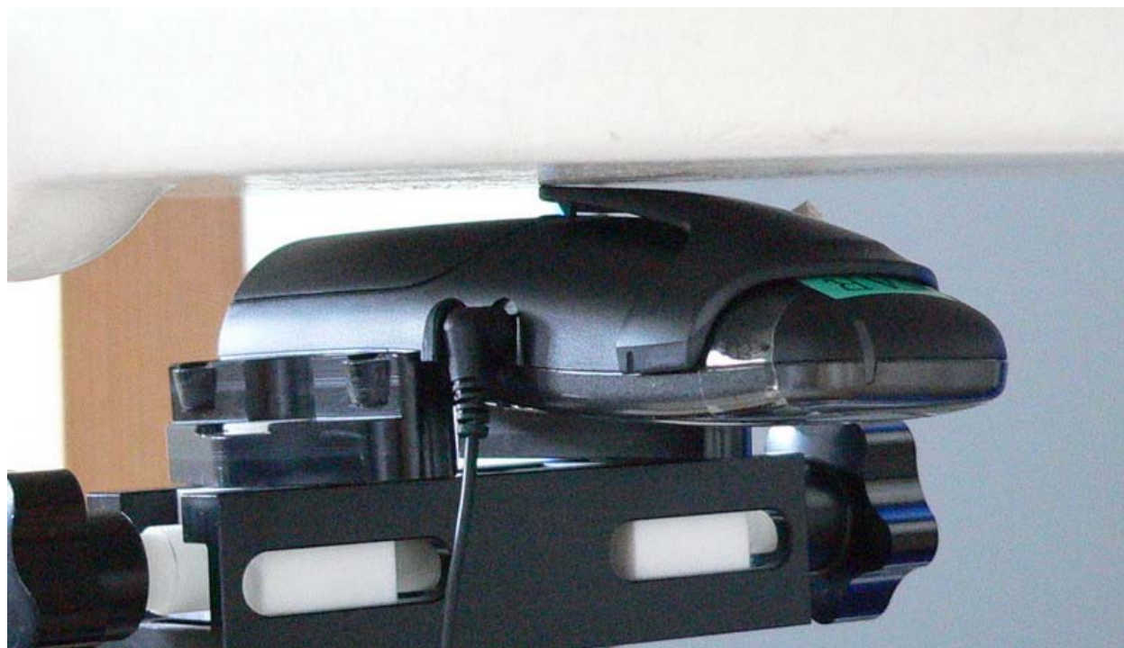
Fig.21: Body worn, position 1, antenna 1 and antenna 2, with belt clip and headset, antennas towards the phantom.
