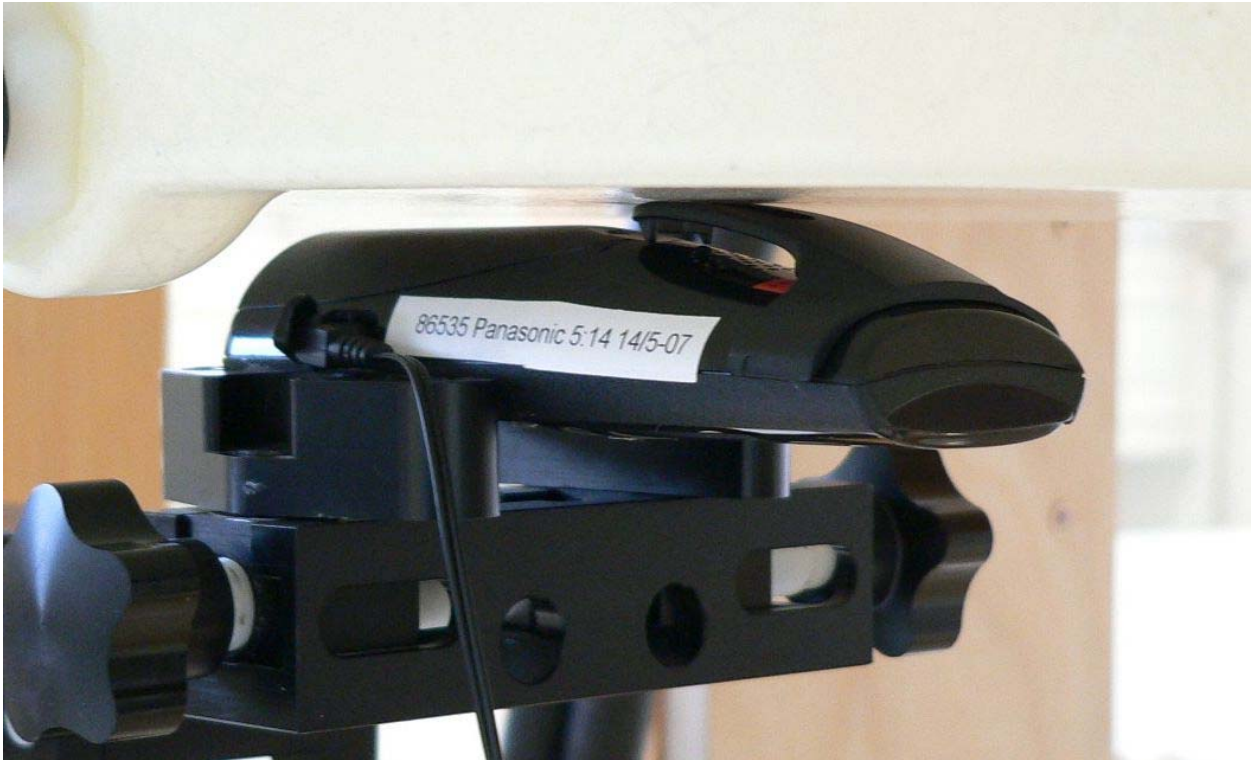
Fig. 8: Body worn, position 2 with belt clip and headset, display towards the ground.
