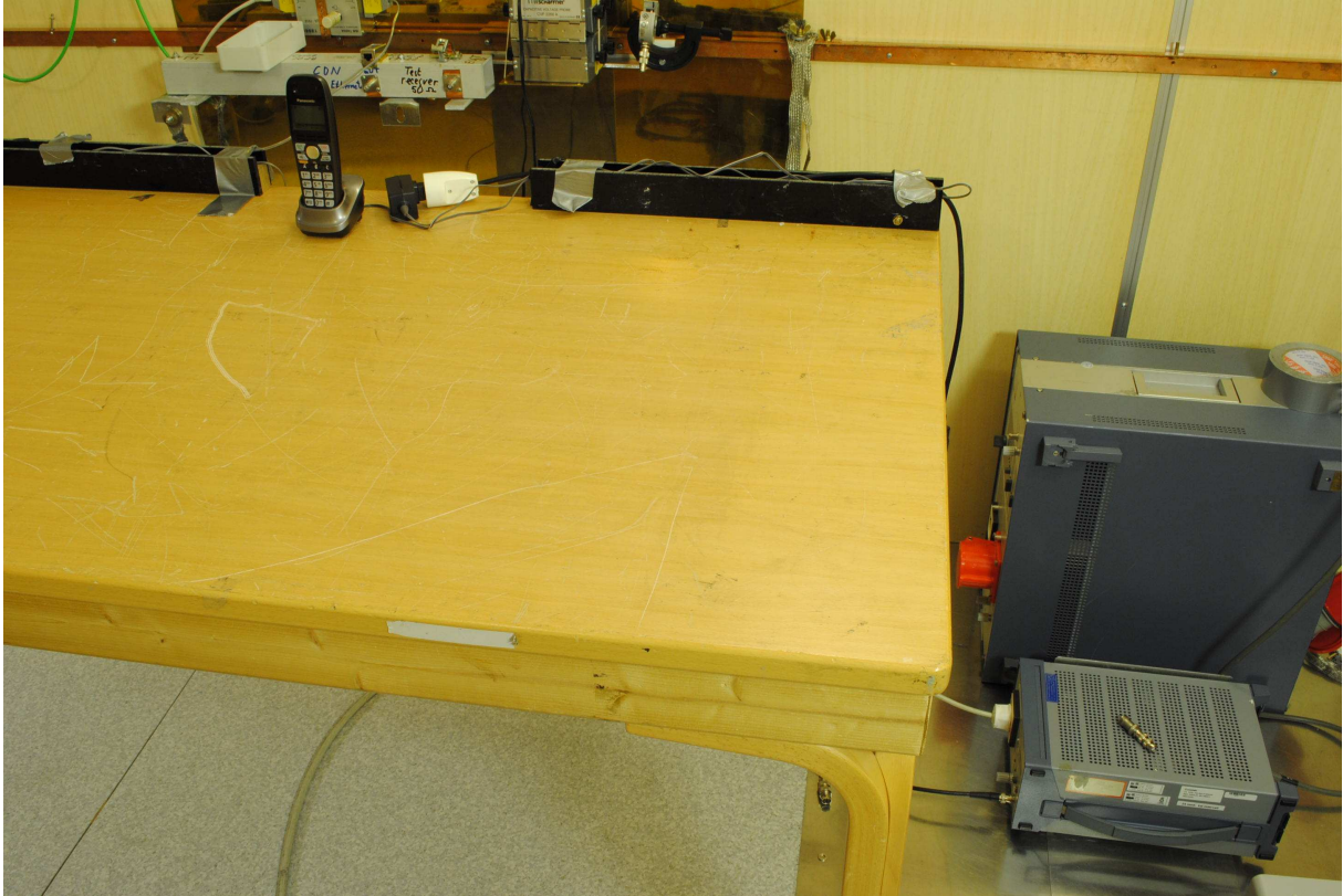
Power line Conducted Emissions Test Set-up
