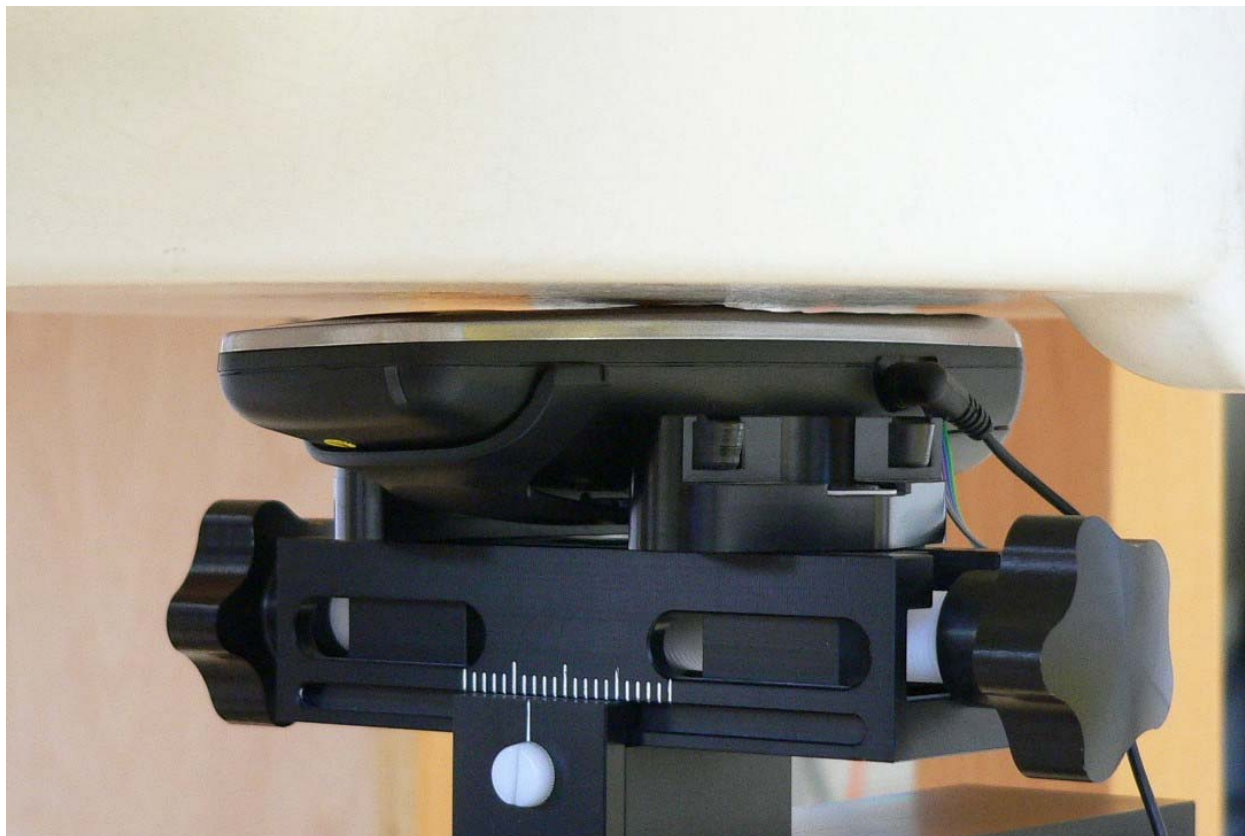
Fig.22: Body worn, antenna 1 or antenna 2, with belt clip and headset, display towards the phantom.
