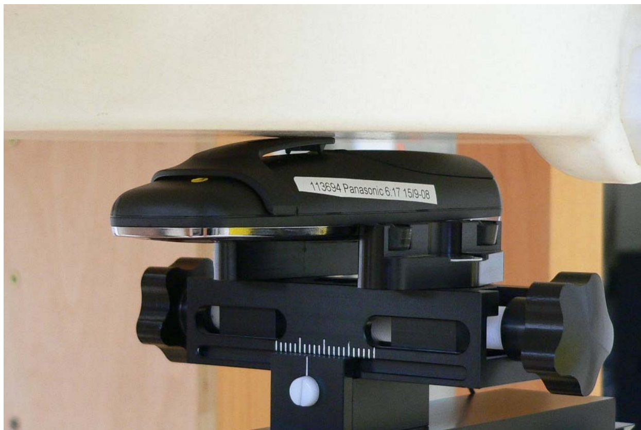
Fig.23: Body worn, antenna 1 or antenna 2, with belt clip and headset, display towards the ground.
