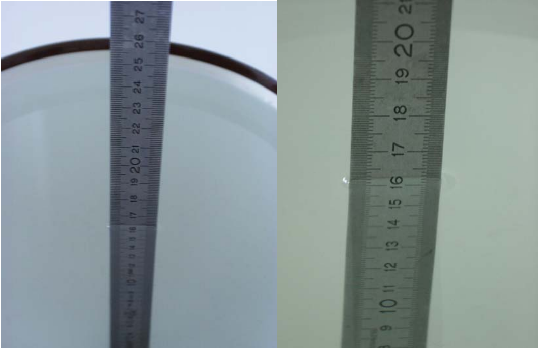
Fig. 22: Liquid depth for GSM 1900 Head and Body measurements.
