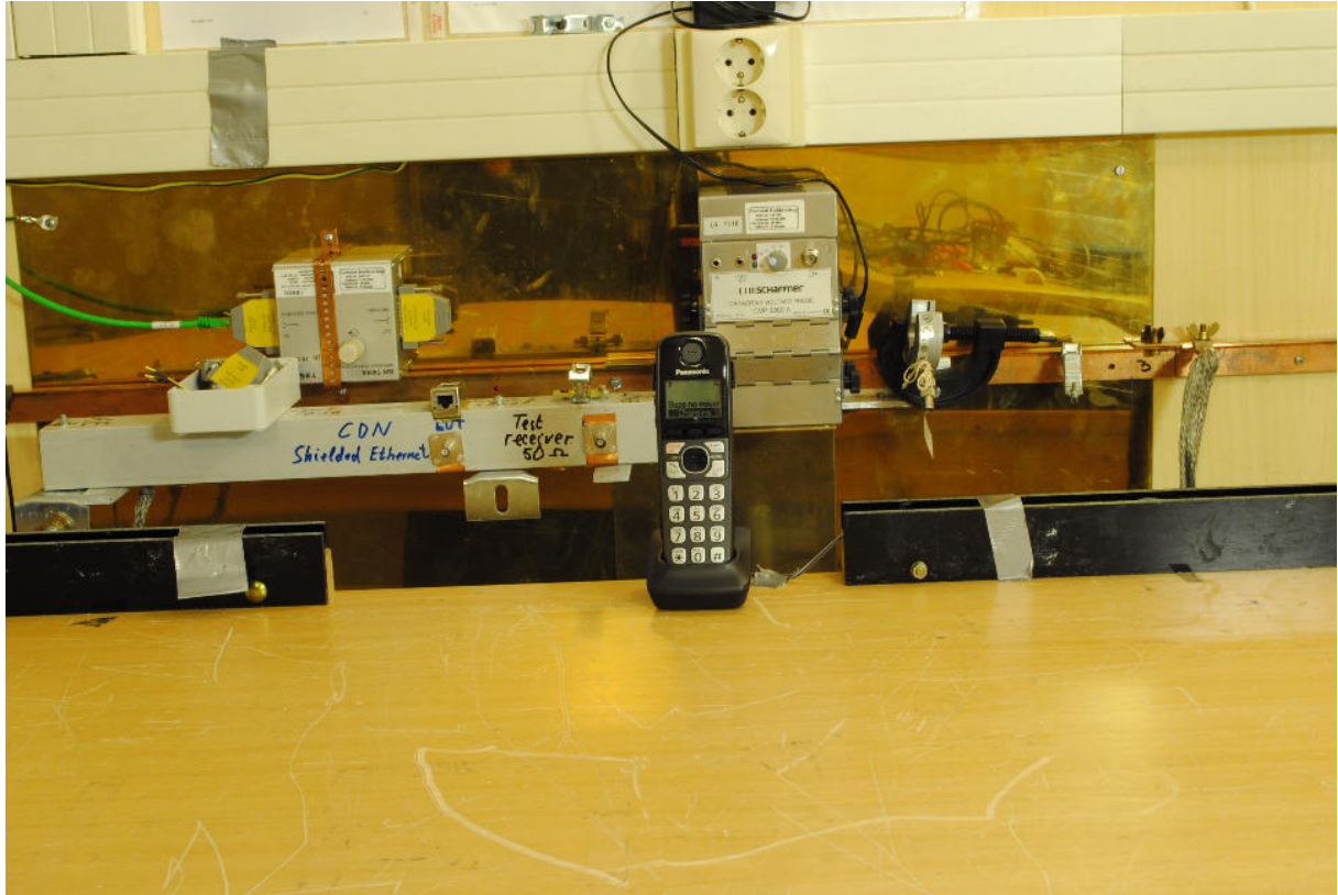
Power line Conducted Emissions Test Set-up
