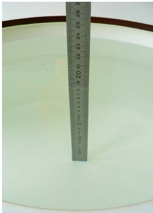
Fig. 23: Liquid depth for 1900 Body worn measurements
