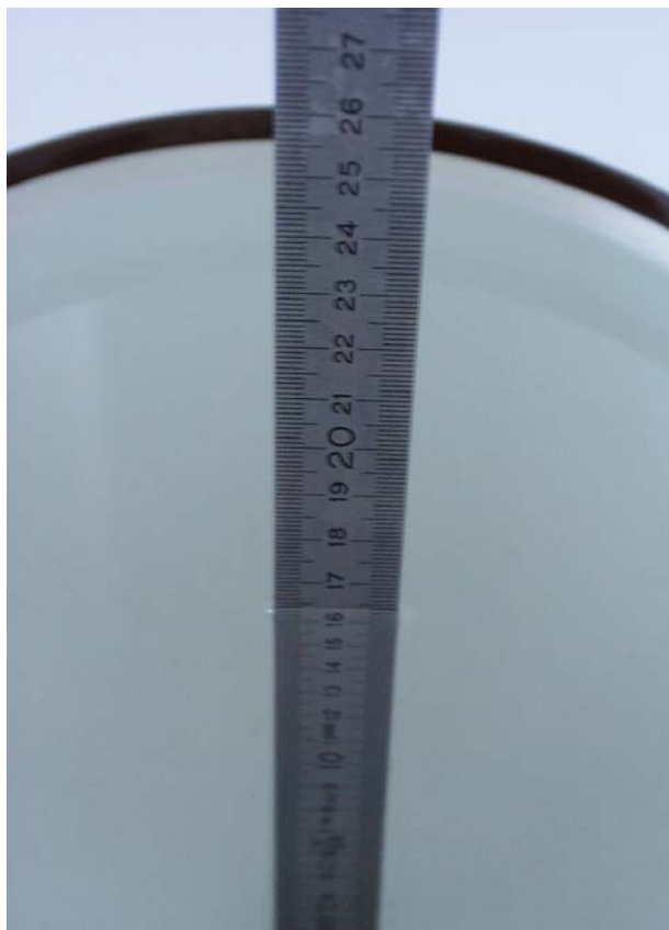
Fig. 22: Liquid depth for 1900 MHz Head measurements
