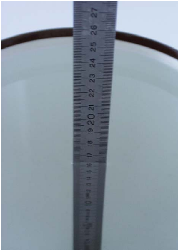
Fig. 17: Liquid depth for 1900 MHz Head measurements
