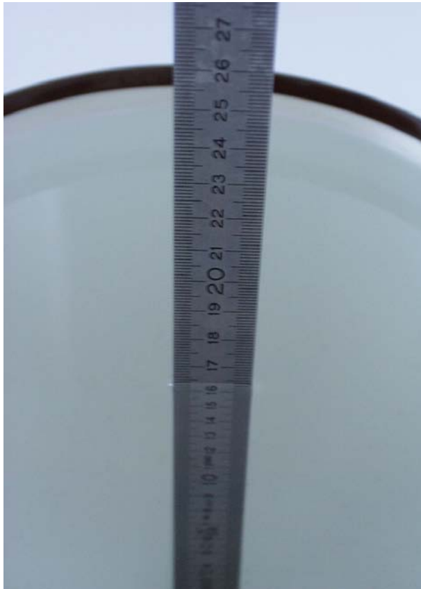
Fig. 17: Liquid depth for 1900 MHz Head measurements
