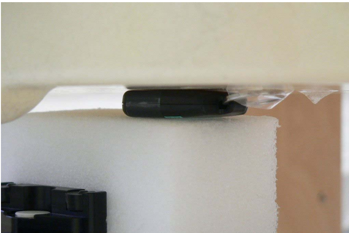
Fig. 14: Body worn configuration for the Panasonic KX-TGA20, back of the device towards the phantom.
