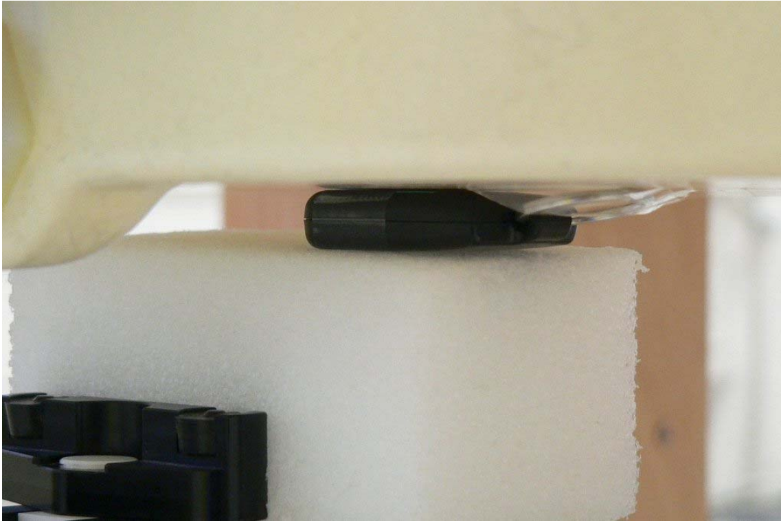
Fig. 13: Body worn configuration for the Panasonic KX-TGA20, front of the device towards the phantom.
