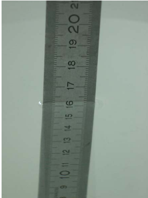
Fig. 15: Liquid depth for 1900 MHz head measurements.
