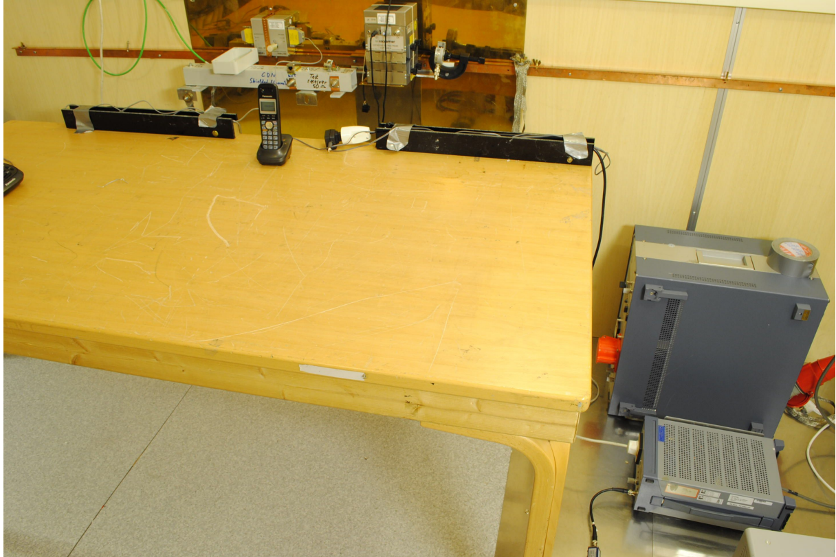
Power line Conducted Emissions Test Set-up
