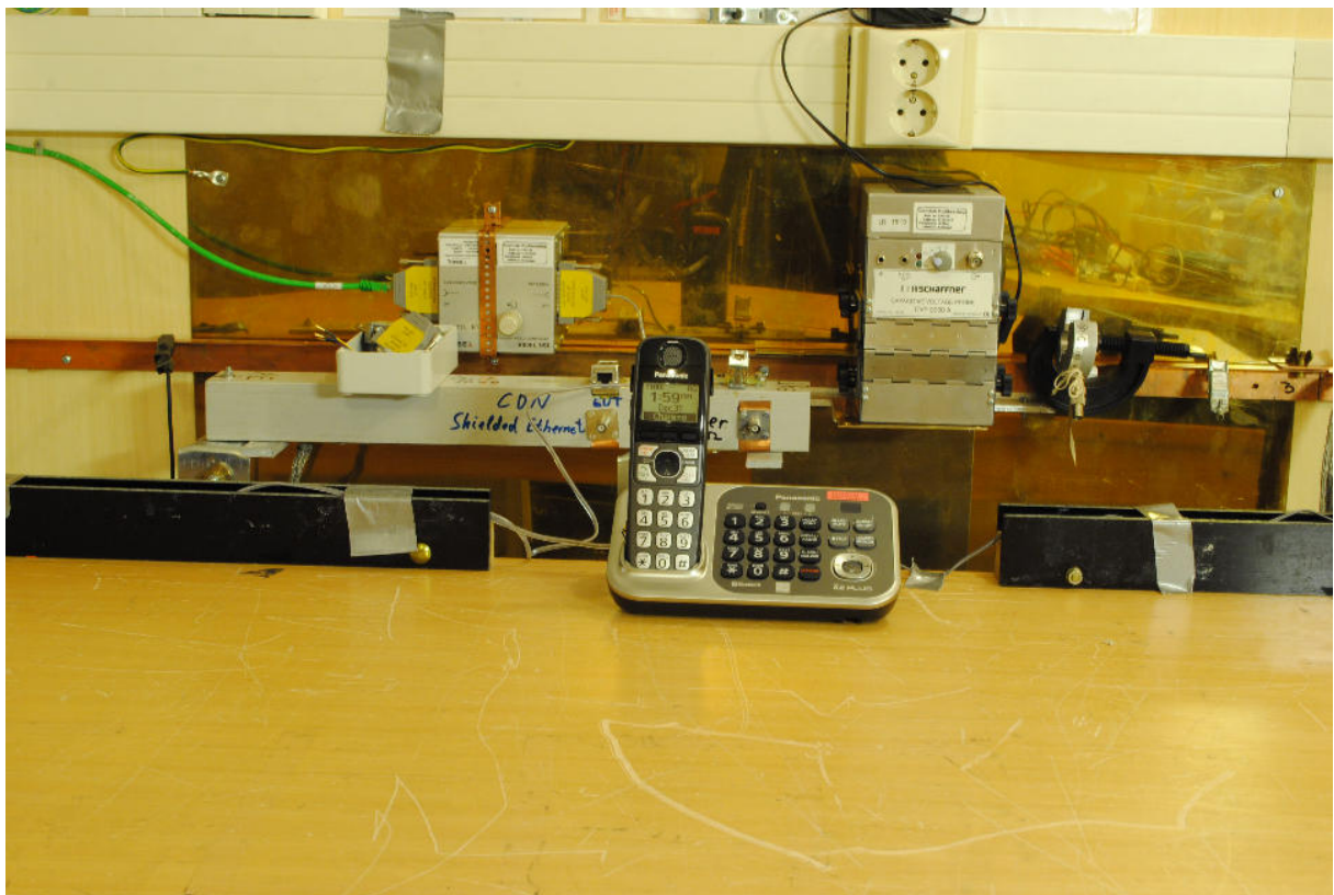
Power line Conducted Emissions Test Set-up
