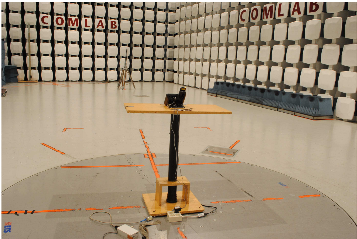
Radiated Emissions Test Set-up
