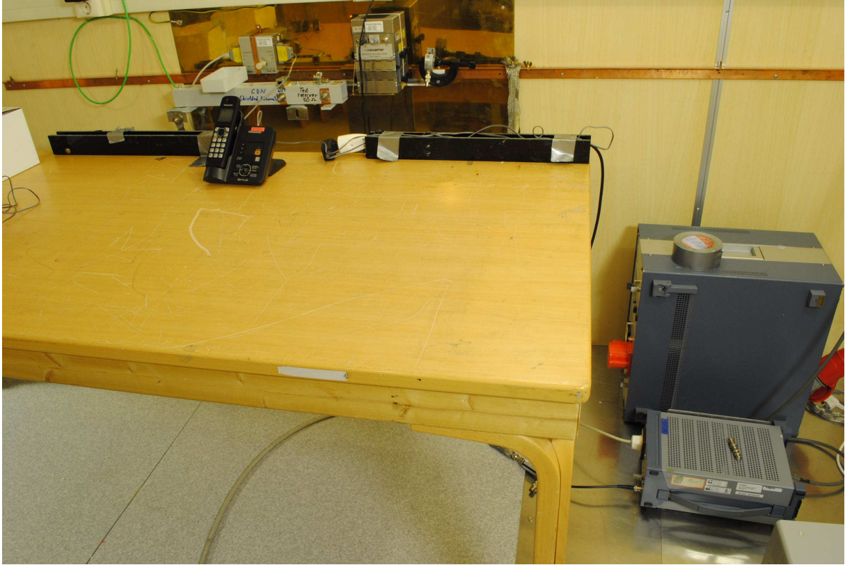
Power line Conducted Emissions Test Set-up
