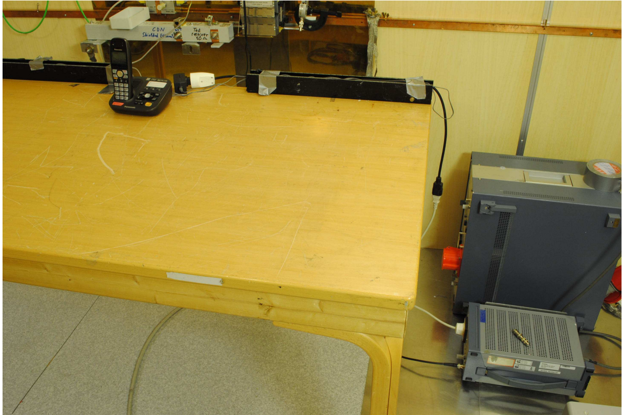
Power line Conducted Emissions Test Set-up
