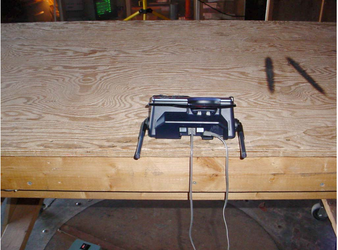
Transmitter/Receiver Radiated Emissions at 3 Metres Base Unit (Antenna parallel to ground plane)
