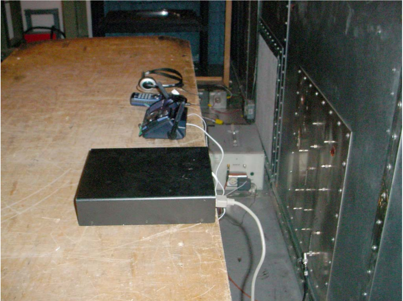
AC Power Line Conducted Emissions (Side View)
