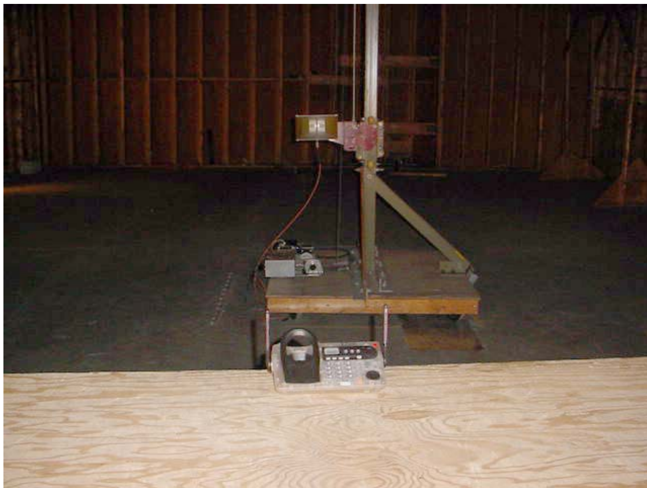
Transmitter Radiated Emissions at 3 Meters Base Unit (Antenna perpendicular to ground plane)
