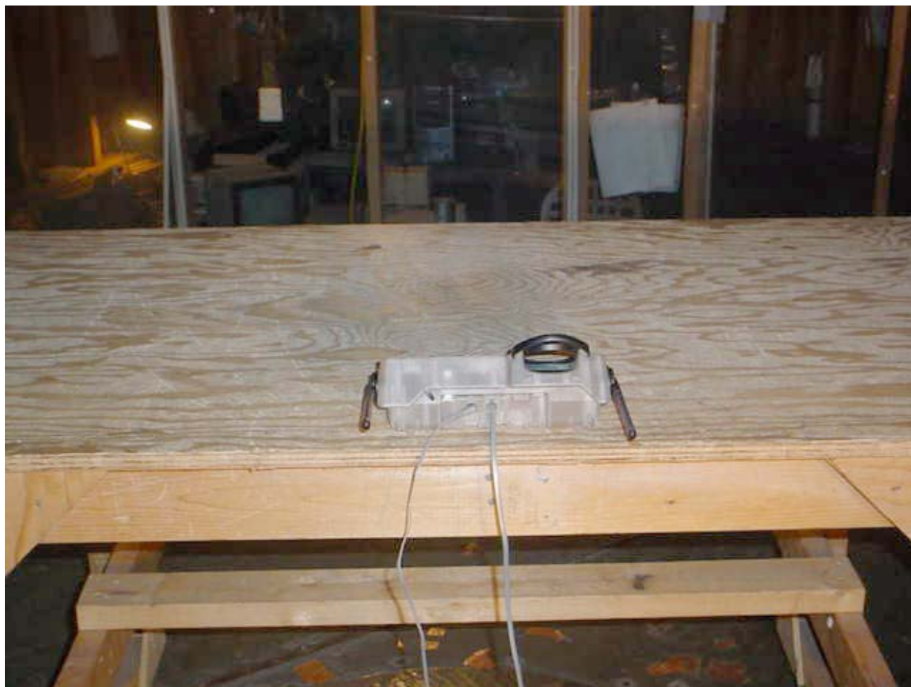
Transmitter Radiated Emissions at 3 Meters Base Unit (Antenna parallel to ground plane)
