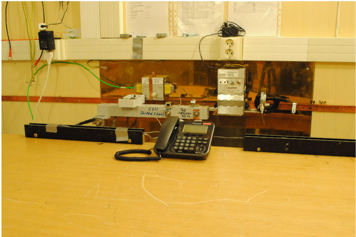
Power line Conducted Emissions Test Set-up
