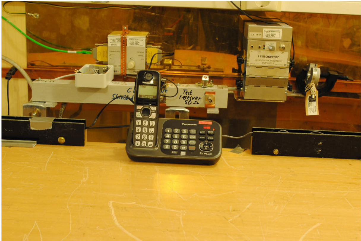
Power line Conducted Emissions Test Set-up
