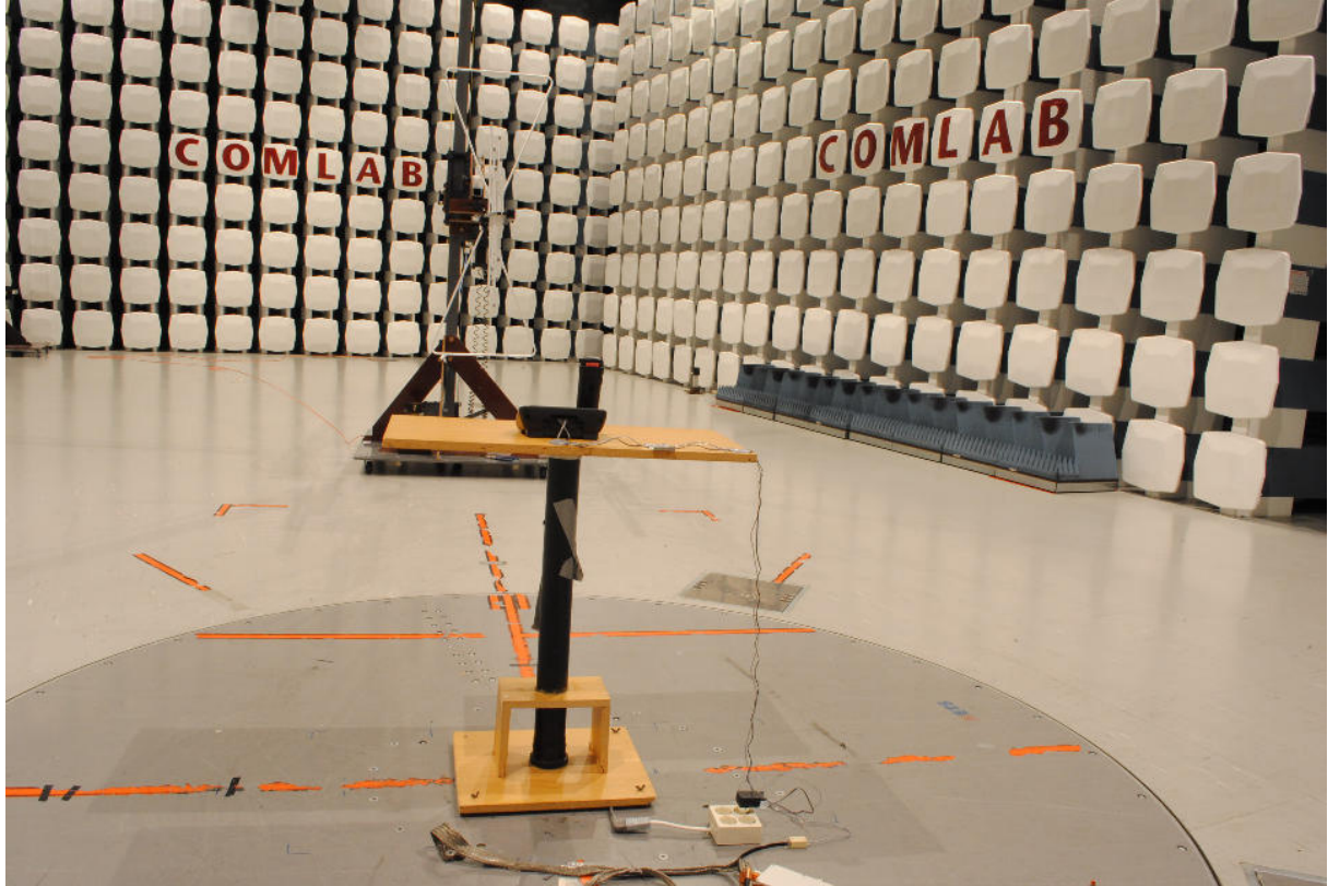
Radiated Emissions Test Set-up
