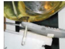
Fig. 14 Head SAR Test Setup
