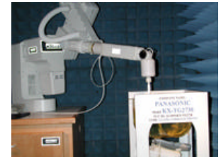
Fig. 1 SAR Test Setup
