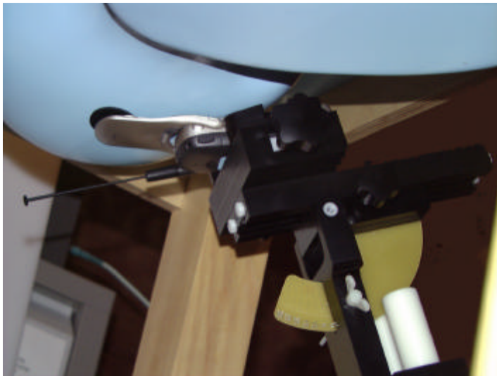
Fig 11. Sample of Handset Alignment with the Ear Canal of the Phantom
