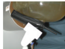
Fig. 14 Head SAR Test Setup
