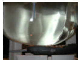
Figure 14.5 Right Head SAR Test Setup -- Cheek / Touch Position --
