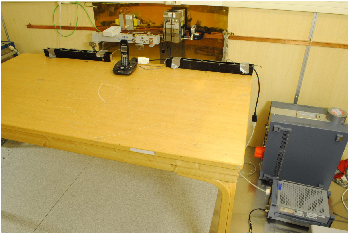
Power line Conducted Emissions Test Set-up
