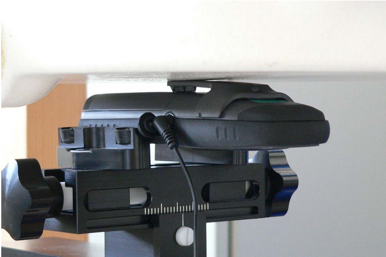
Fig.21: Body worn, with belt clip and headset, antenna towards the phantom.
