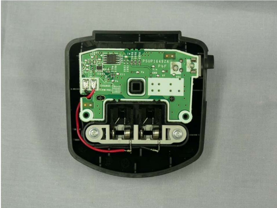
Internal view of battery charger for KX-TD7696
