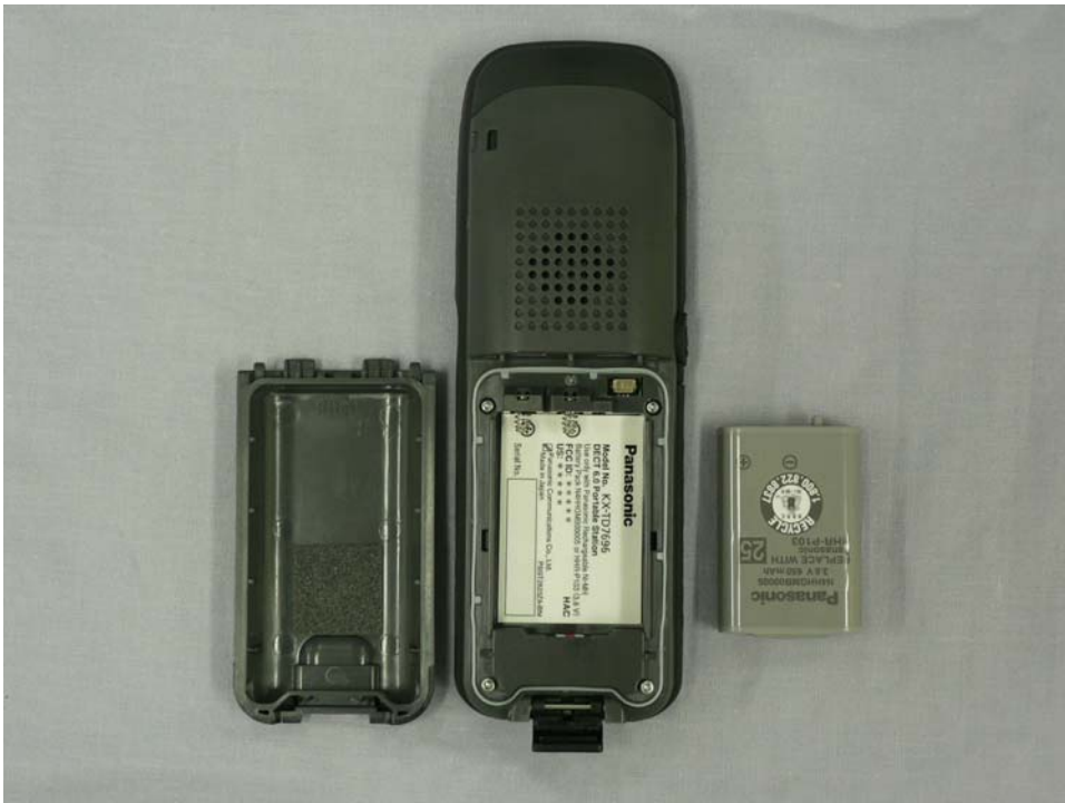
KX-TD7696 Rear view of handset (battery cover & battery removed)
