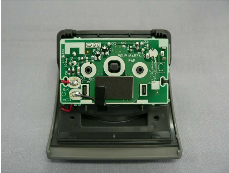
Internal view of battery charger for KX-TD7684
