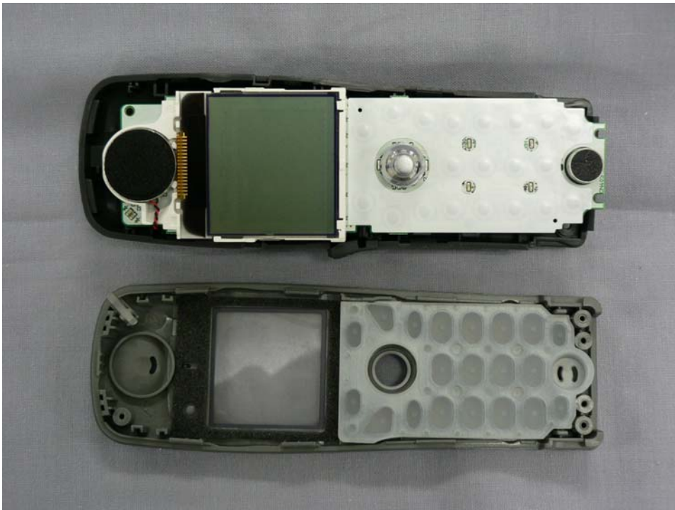
KX-TD7684 Internal view of handset
