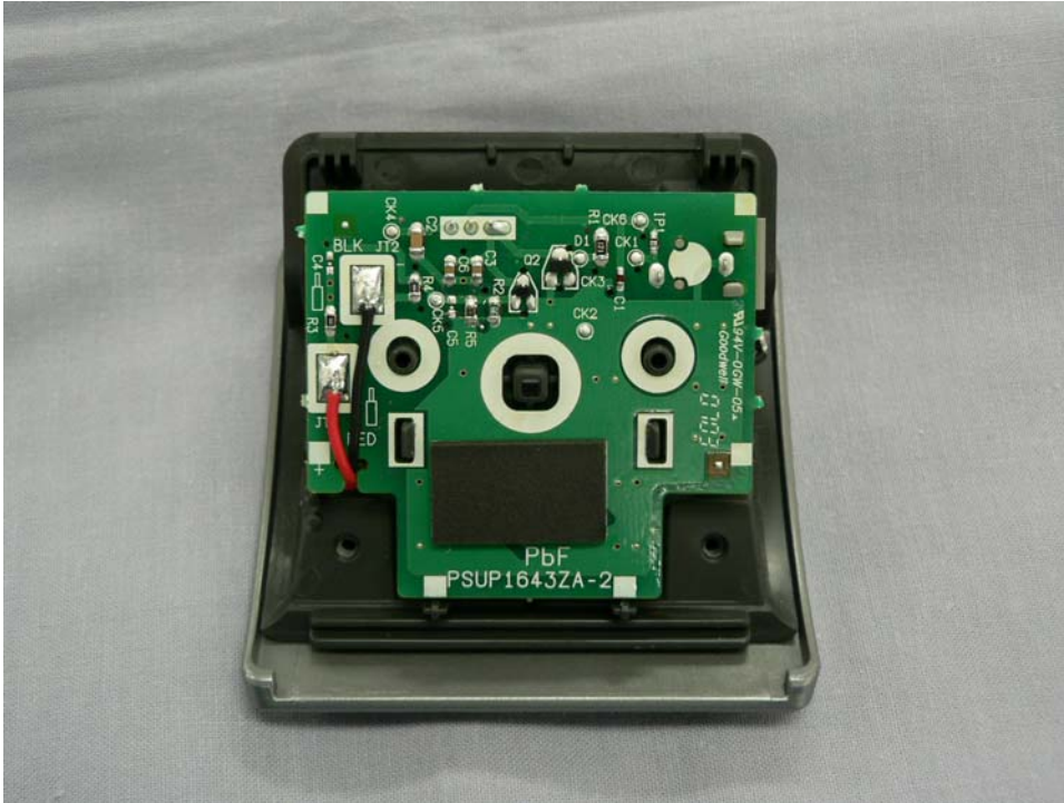
Internal view of battery charger for KX-TD7694
