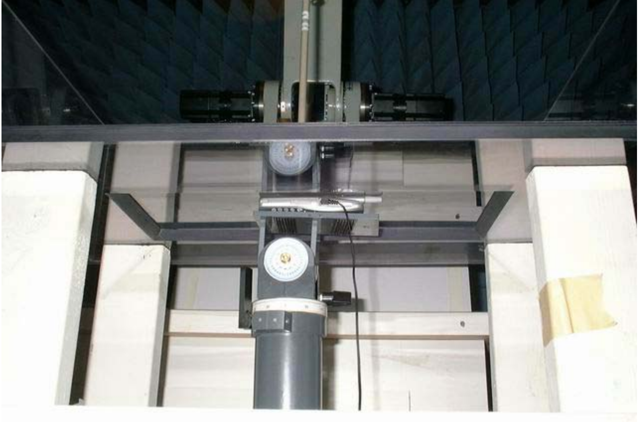
< Display faced outward from the phantom with headset(M/N:KX-TCA88) – Overview >
