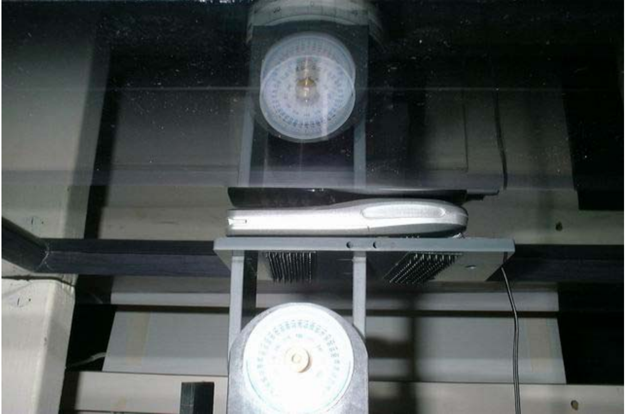
< Display faced inward to the phantom with headset(M/N:KX-TCA88) – Close-up View >
