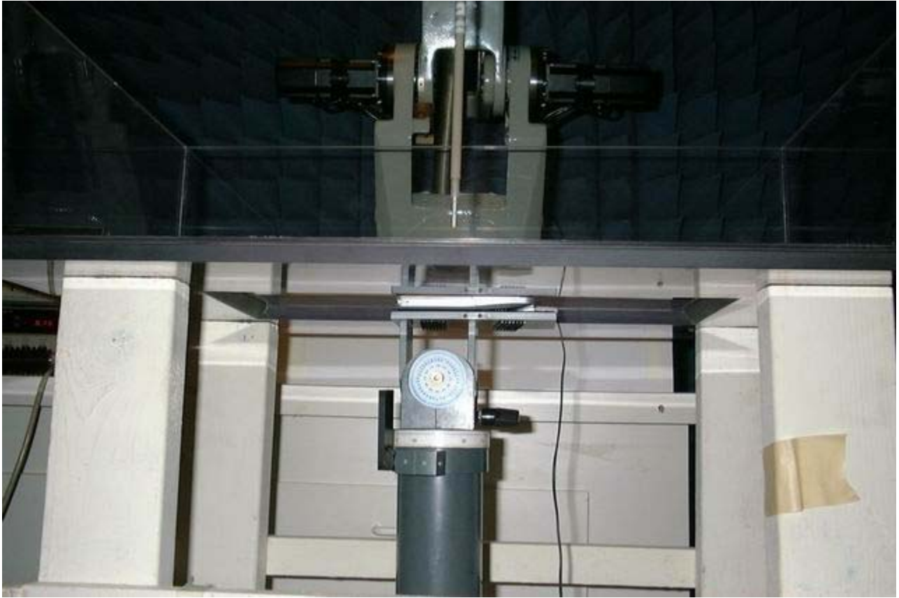
< Display faced inward to the phantom with headset(M/N:KX-TCA88) – Overview >
