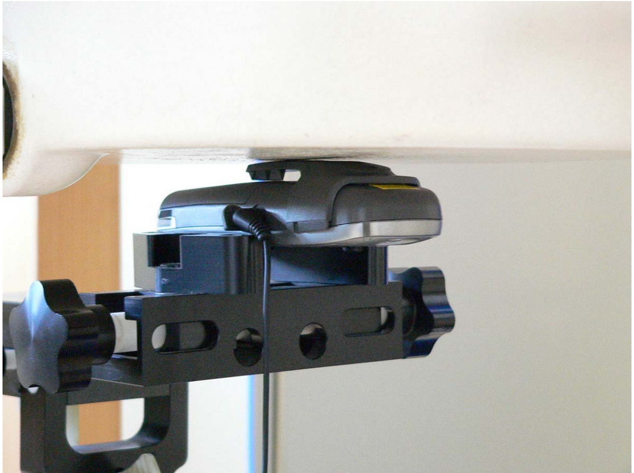
Fig. 20: Body worn, position 1, with belt clip and headset, antennas towards the phantom.
