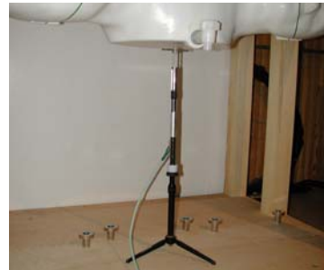
Figure 12.1 Dipole Validation Test Setup
