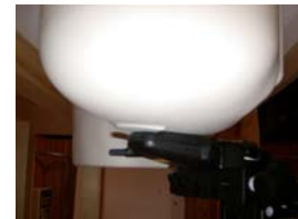
Figure 14.3 Head SAR Test Setup -- Right-Touch --
