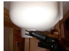
Figure 14.5 Head SAR Test Setup -- Right-Tilt --
