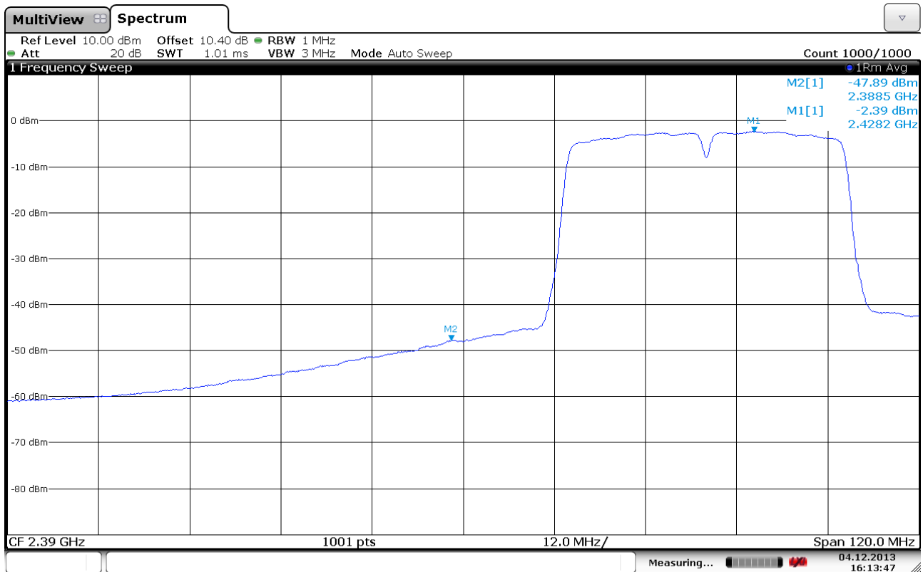
Lower Band Edge, Conducted, Average, 2422 MHz, 802.11n, MCS7, 40MHz BW
