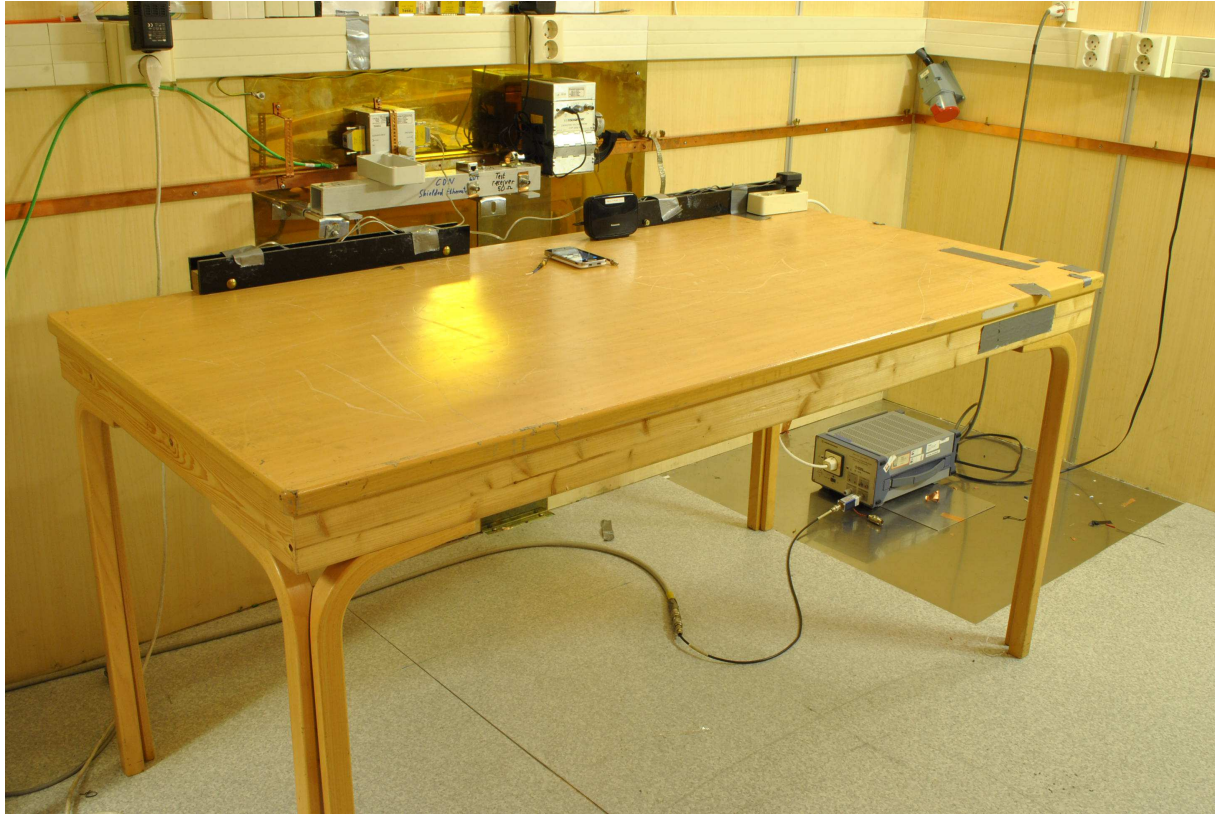
Power line Conducted Emissions Test
