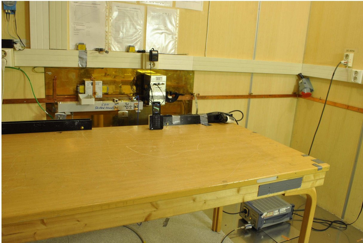
Power line Conducted Emissions Test
