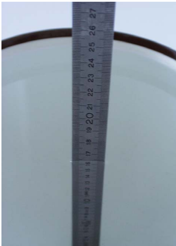
Fig. 17: Liquid depth for 1900 MHz Head measurements
