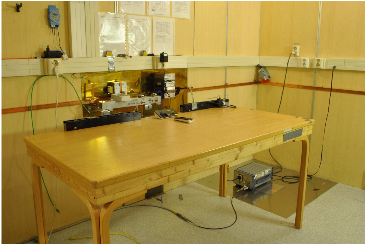
Power line Conducted Emissions Test
