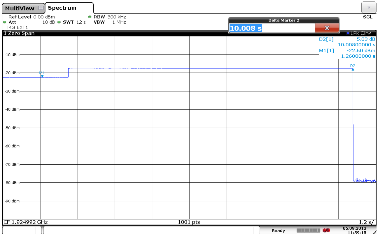
8.2.1c) Transmission Time After Loss of Acknowledgements
