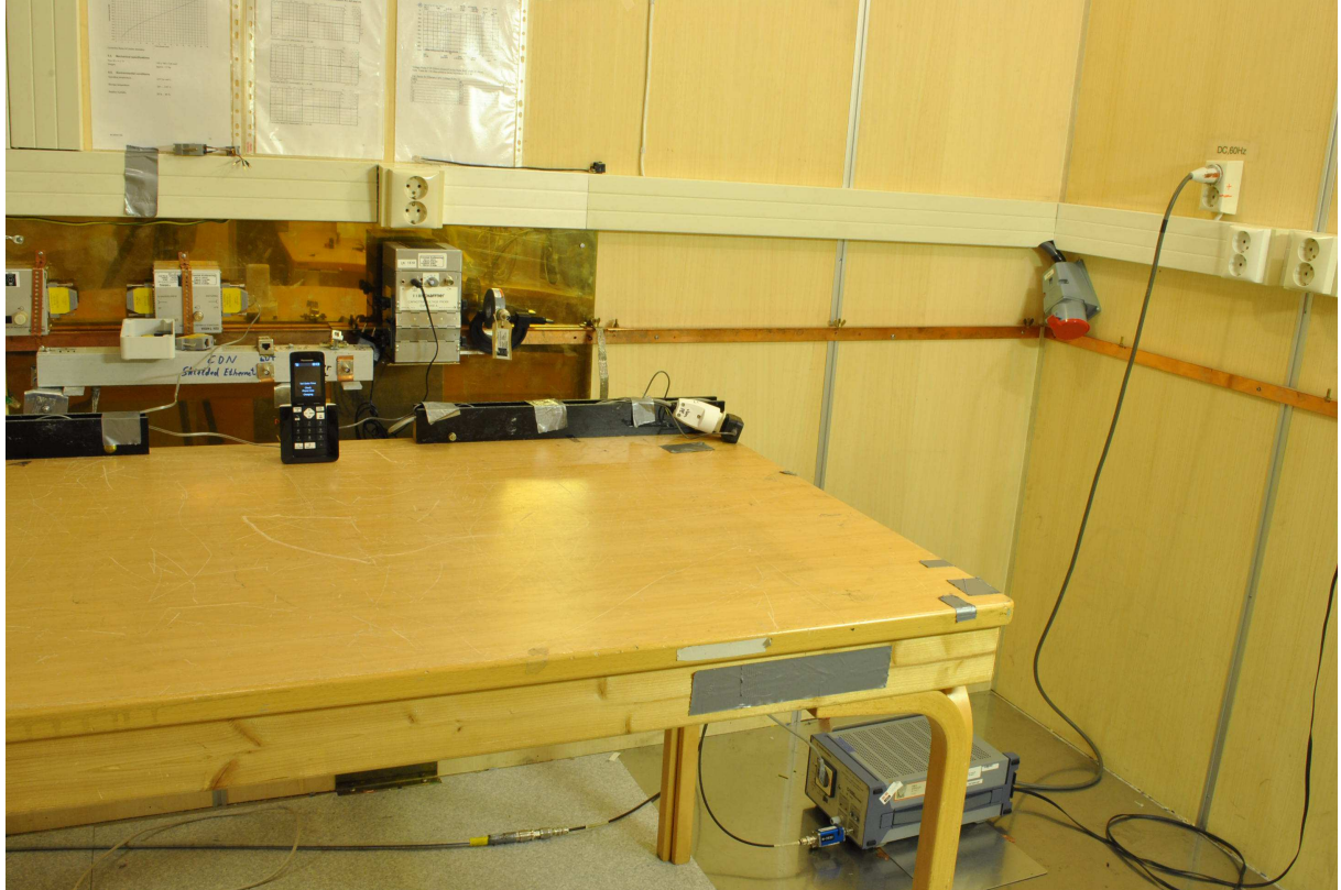
Power line Conducted Emissions Test
