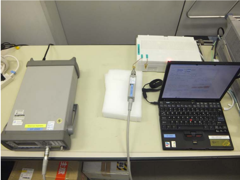
Photograph 1: Set-up for Conducted Emissions at Antenna Port
