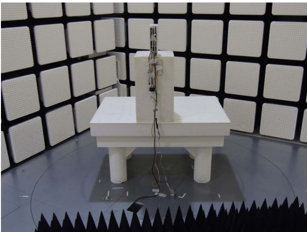
Photograph 5: Set-up for Radiated Emission, Above 1GHz, EUT Configuration Y-Axis of Transmitter, Rear View
