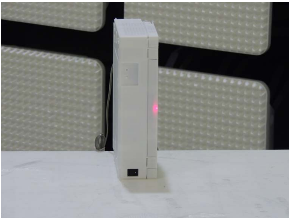
Photograph 7: Set-up for Radiated Emission, EUT Configuration Y-Axis
