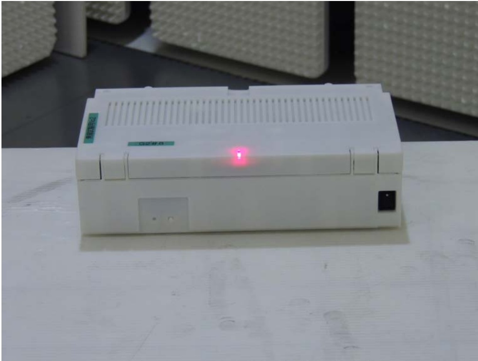
Photograph 6: Set-up for Radiated Emission, EUT Configuration X-Axis
