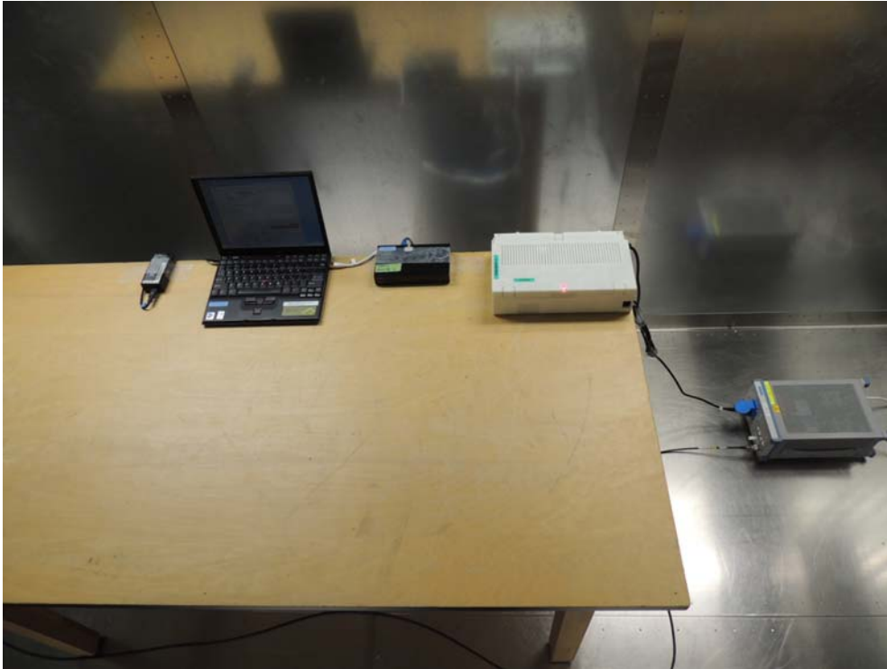
Photograph 8: Set-up for AC Power Line Conducted Emission of Transmitter, Front View
