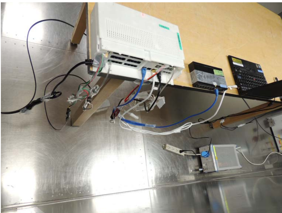
Photograph 9: Set-up for AC Power Line Conducted Emission of Transmitter, Rear View
