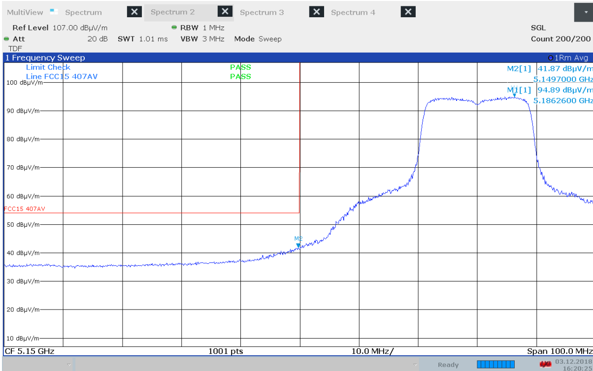
Band Edge, 5150 MHz, Ch036, 802.11n MCS0, EUT V (Max: HP), Average
